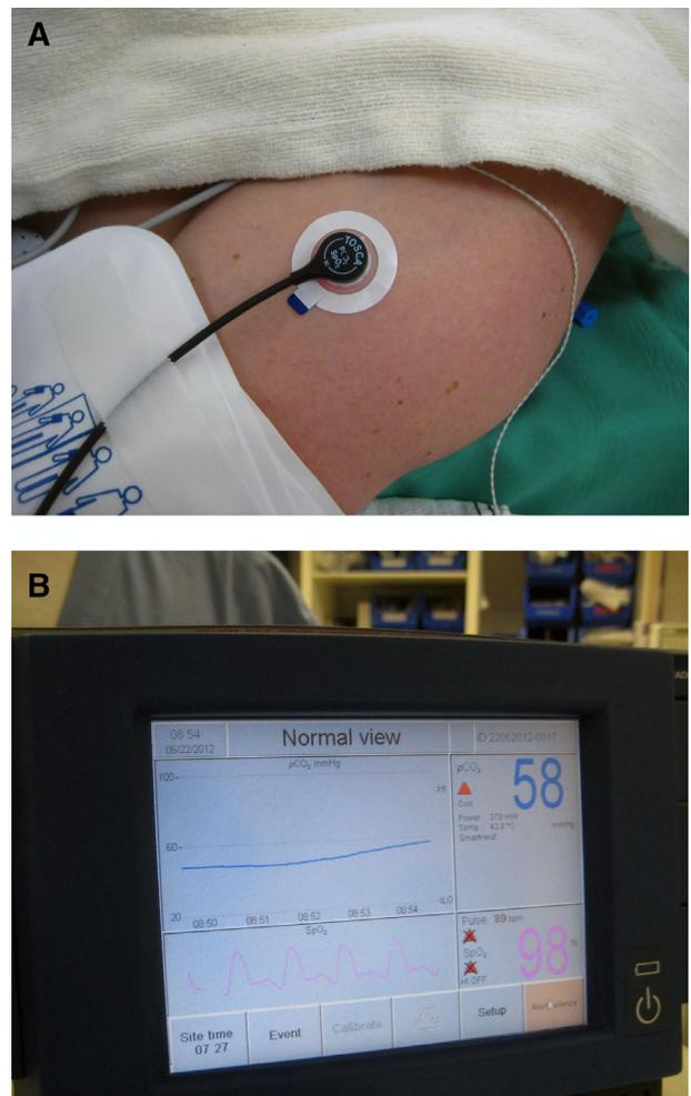
Fig. 4. (A) A transcutaneous CO<sub>2</sub> sensor, and (B) a transcutaneous CO<sub>2</sub> monitor.
