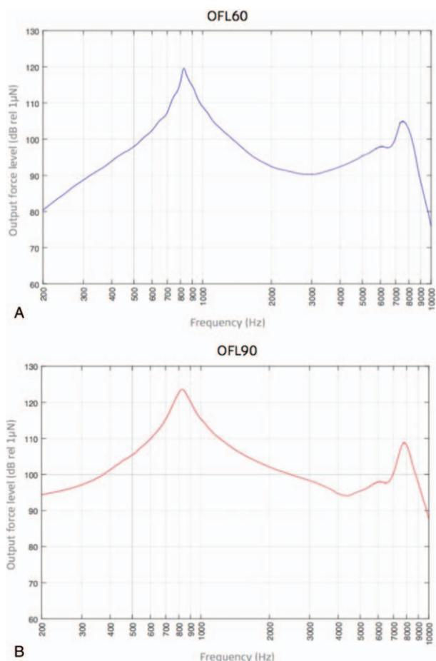
**FIG. 3.** Output force level (OFL) (in dB rel 1  $\mu$ N) frequency response (in Hz) for a specific input sound pressure level measured on the skull simulator SKS10 with the adhesive test device. A, Represents the OFL at 90 dB SPL and (B) the OFL at 60 dB SPL.
